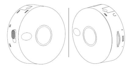
On the rear of the machine, you'll see a large black wheel/knob assembly. This is the control center for your audio system. The largest knob/wheel, taking up the entire outer rim of the assembly, is your volume control. Spin to adjust volume up/down. You'll also see a smaller spin wheel on the side labeled BASS, which is your bass control. Spin to adjust. Lastly, there is an on/off toggle switch on the side as well for your audio systems power control.
