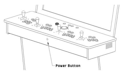
After connecting your arcade's power cable from the wall to the arcade, locate the black pushbutton mounted on the front of your arcade as shown above. To turn your arcade on, simply press this button inwards. Once pressed, the internal PC inside your arcade will power on as well as your LED Marquee, LED pushbuttons and monitor.
