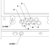
Directional Pad (D-PAD) = Joystick control X, Y, Z, A, B, C = Buttons 1, 2, 3, 5, 6 & 3 START = Player START 3. The Super Nintendo Entertainment System had a Four-button controller (Y, X, B, A), two shoulder bumper buttons (LB, RB), a SELECT & START button, and an UP/DOWN/LEFT/RIGHT directional pad, as shown below. The corresponding button configuration for this system on your arcade is:
