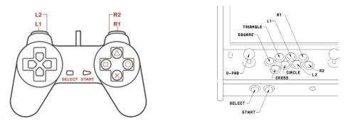
Directional Pad (D-PAD) = Joystick control SQUARE, TRIANGLE, CROSS, CIRCLE = Buttons 1, 2, 5, 6 L1, R1, L1, L2 = Buttons 3, 4, 7, 8 SELECT, START = Player COIN, START
